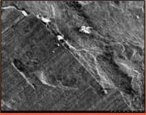
Too thick of diffusion zone leads to chipping, flaking, and cracking of the FNC
