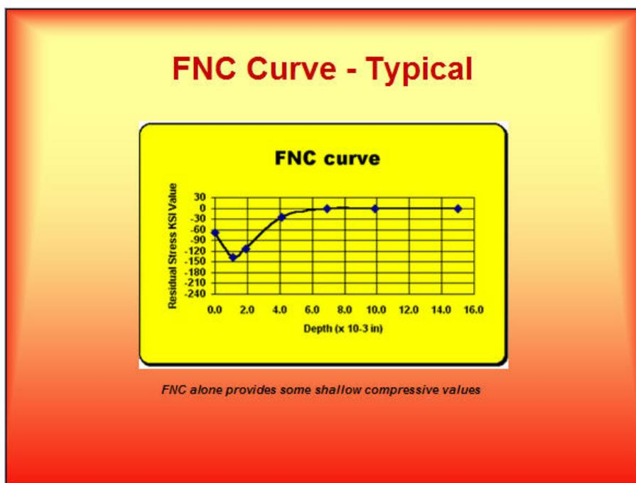
It is this diffusion zone and compound layer that provide protection against soldering of aluminum for die casting & extruding tooling, increased wear resistance, and protection against corrosion, while providing an increase in the fatigue strength of the steel from compression.
